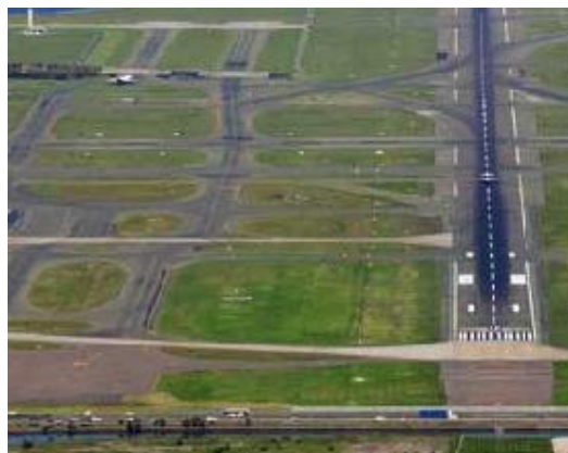
Figure 3.4 Typical example of terrain category 2.
